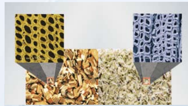
chip structure before impregnation chip structure after impregnation
